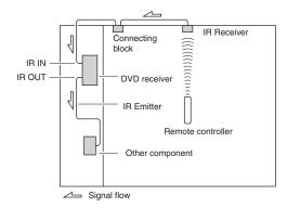
The IR emitter should be connected to the DVD receiver's IR OUT jack, as shown below.
